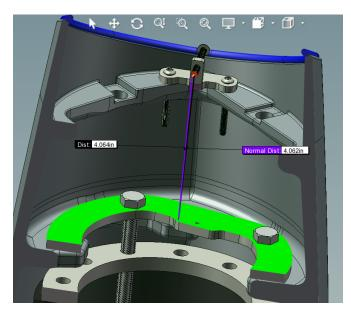
3D model of assembled bollard showing plate cap screw (red) and location of LED light (green). Light not shown for clarity.
