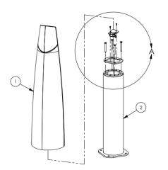
1) bollard sleeve and acrylic lens, 2) internal post, A) lighting assembly and connector ring (below).
