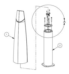
1) bollard sleeve and acrylic lens, 2) internal post, A) lighting assembly and connector ring (below).
