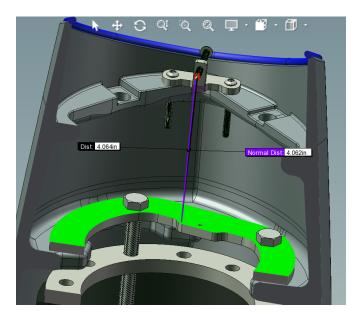
3D model of assembled bollard showing plate cap screw (red) and location of LED light (green). Light not shown for clarity.
